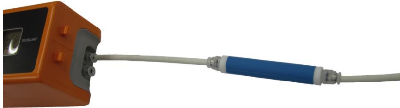
Figure 4. Sampling Port Connection
