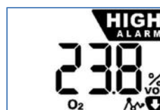
Alarm Value Occurred Display
